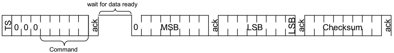
Figure 6 Overview of Measurement Sequence (TS =Transmission Start)
