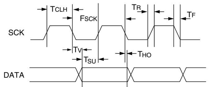
Figure 9 Timing Diagram
