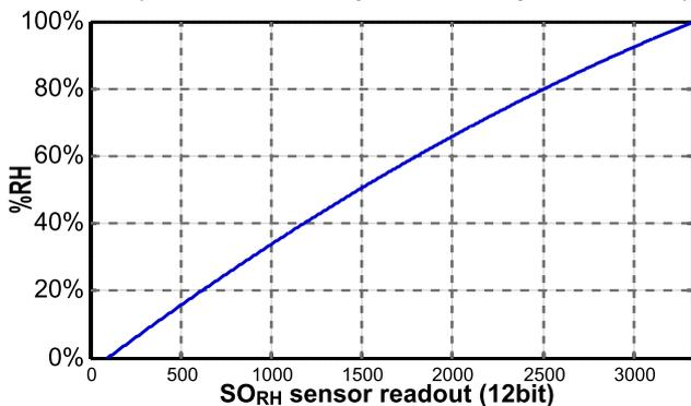
**Figure 10** Conversion from SO<sub>RH</sub> to relative humidity
